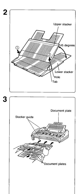
Connect the tabs of the Lower stacker to the holes of the Upper stacker.
