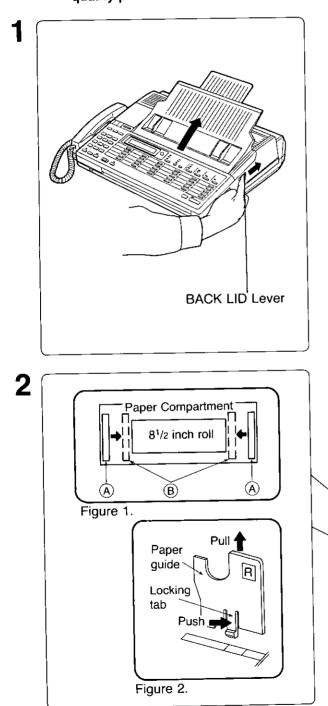
Slide the back lid lever in the direction of the arrow to open the cover.
